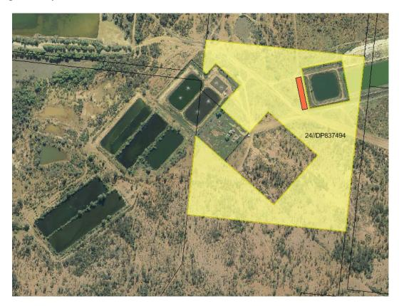
The red rectangular area shown on the above map indicates the area where Cobar Shire Council as part of the Infrastructure NSW funding for the Sewerage Projects (Chlorination Facility) is going to be constructing an advanced biological tertiary filter system (reed beds).
